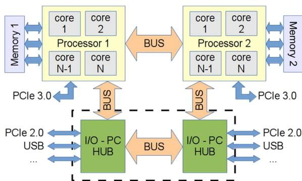
Fig. 1. Block diagram of a generic NUMA architecture
