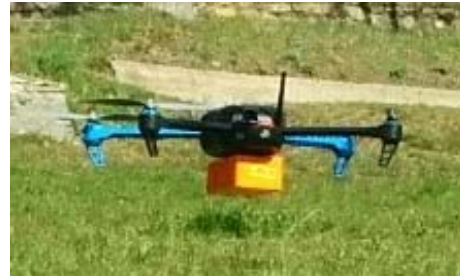
Figure 2. UAV and RFID reader
