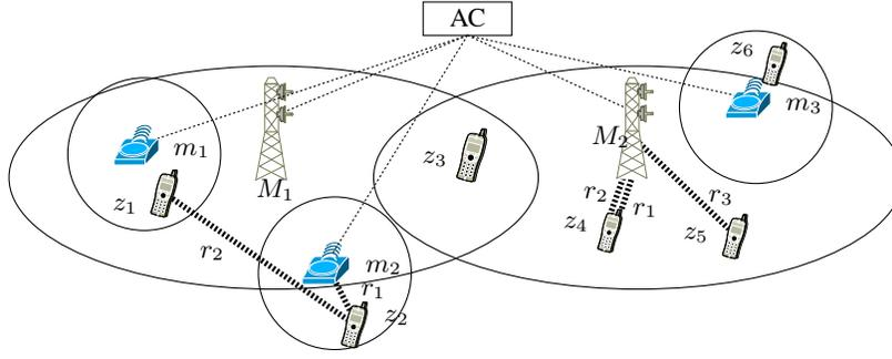
Fig. 1. An example scenario. UEs are denoted by  $z_1, \dots, z_6$ , macroBSs by  $M_1, M_2$  and microBSs by  $m_1, m_2, m_3$ . Solid lines denote coverage areas. Dotted lines correspond to RBs used by a pair of endpoints.
