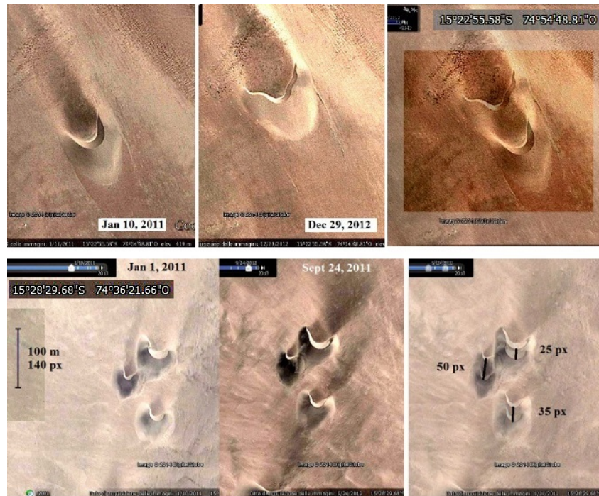
Figure 1 - Moving dunes in the time series of Google Earth images (coordinates: 15^{\circ}22'55.58''S , 74^{\circ}54'48.81''W , and 15^{\circ}28'29.68''S , 74^{\circ}36'21.66''W ; Courtesy Google Earth). Using GIMP, we can measure the speed of dunes. Two images, recorded at different time, are combined in the same image. In fact, GIMP allows laying an image on the other [8]. Then, using a tool of GIMP, the pair of compasses, we can measure the displacement of dunes in pixels. Since from Google Earth, we know distances on the ground, we can convert pixels in meters. In the image on the right, we can see three dunes, the smaller is moving faster than the other two [1].
