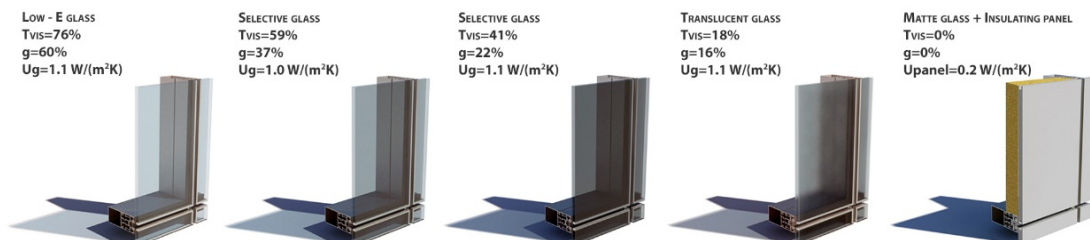
Fig. 1. Characteristics of the five typologies of glazing used in the parametric study.
