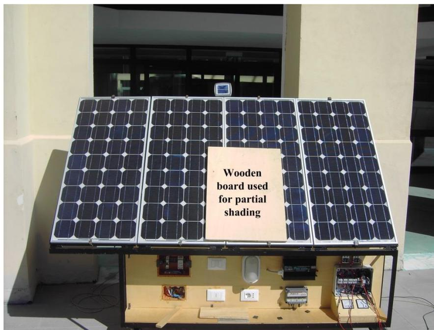
**Figure 5.21** – PV array is partially shaded with the help of wooden board
