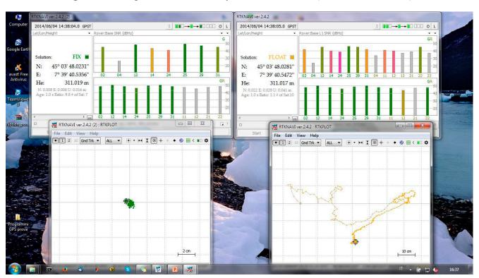
Figure 4. Float positions obtained by the NVS receiver (RTKNAVI window).
