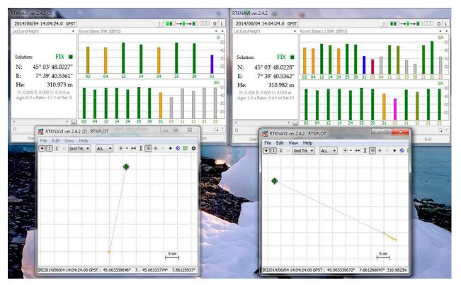
Considering these experiments, we have fixed the ambiguities using a "ratio" equal to 3 both for the GPS and GLONASS constellations using a "continuous" method. This means that the software verifies whether the fix of the phase ambiguity is correct at each epoch. Moreover, we have chosen a cut-off angle of 10° in order to neglect the signals coming from satellites with low elevations (that are very noisy).
