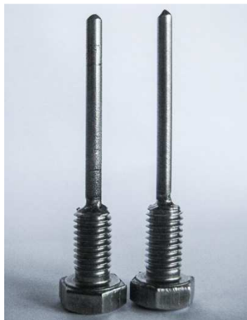
Figure 13 Electrodes: Co-Cr alloy cathode (on the left) and Ni-Fe alloy anode.
