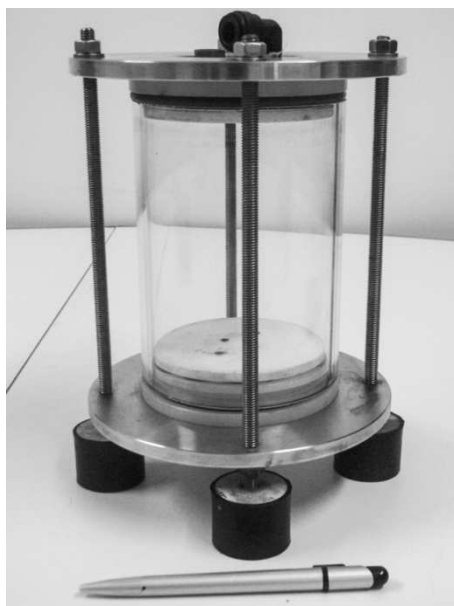
Figure 12 Electrolytic cell: glass cylindrical container sealed with Teflon lids.
