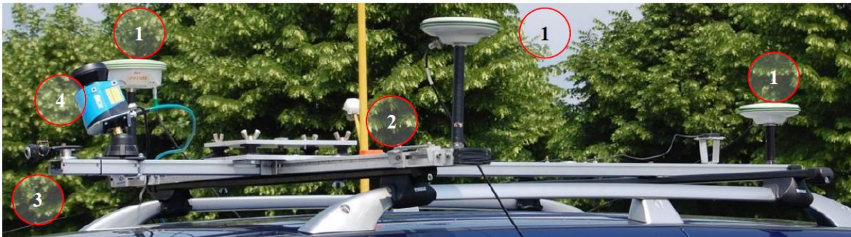
Figure 4.2 - The new, low cost prototype MMS with sensors. (1) GNSS receivers Leica GX1230+ (2) GPS/IMU Xsens MTi-G, (3) Logitech Quickcam Pro 9000 webcam, (4) LMS-110 Sick laser scanner
