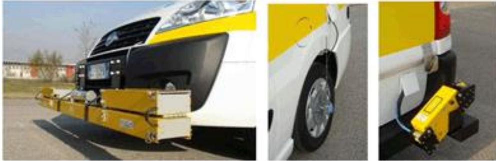
Figure 1.10 – A typical MMV equipped to identify road geometry properties
