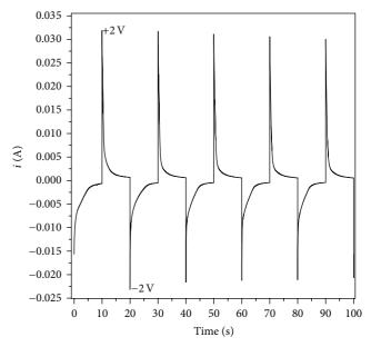
FIGURE 7: Chronoamperometric profile of a WO<sub>3</sub>/PE/V<sub>2</sub>O<sub>5</sub> ECD. Electrodes configuration: WO<sub>3</sub>/ITO/Glass as working electrode and V<sub>2</sub>O<sub>5</sub>/ITO/PET as counter and reference electrode.  $E_1 = -2.0$  V,  $E_2 = +2.0$  V versus V<sub>2</sub>O<sub>5</sub> electrode.  $t_1 = t_2 = 10$  s.
