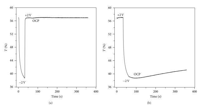
FIGURE 14: Time stability UV-VIS Transmittance measurements at open circuit and fixed wavelength (700 nm) for a WO<sub>3</sub>/PE/V<sub>2</sub>O<sub>5</sub> ECD. Electrodes configuration:WO<sub>3</sub>/ITO/Glass as cathode and V<sub>2</sub>O<sub>5</sub>/ITO/PET as anode. (a) bleached state (E = +2 V versus V<sub>2</sub>O<sub>5</sub> for 10 s); (b) coloured state (E = -2 V versus V<sub>2</sub>O<sub>5</sub> for 10 s).
