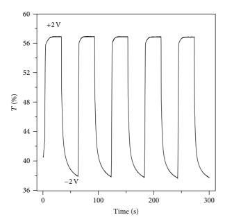
FIGURE 9: Time plot of UV-VIS transmittance at 700 nm during repeated switching between bleached and coloured state for a WO<sub>3</sub>/PE/V<sub>2</sub>O<sub>5</sub> ECD. Electrodes configuration: WO<sub>3</sub>/ITO/Glass as cathode and V<sub>2</sub>O<sub>5</sub>/ITO/PET as anode. Potential program:  $E_1 = +2$  V;  $E_2 = -2$  V (versus V<sub>2</sub>O<sub>5</sub> electrode);  $t_1 = t_2 = 30$  s.
