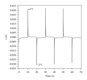
FIGURE 6: Chronoamperometric profile of a WO<sub>3</sub>/PE/ITO ECD device. Electrodes configuration: WO<sub>3</sub>/ITO/Glass as working and ITO/PET as counter and reference electrode.  $E_1 = -2.0$  V,  $E_2 = +2.0$  V versus ITO electrode.  $t_1 = t_2 = 10$  s.
