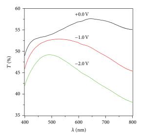
FIGURE 8: UV-VIS transmittance spectra of a complete cell containing  $V_2O_5$  and  $WO_3$  films registered at 0, -1, and -2 V versus  $V_2O_5$  electrode.
