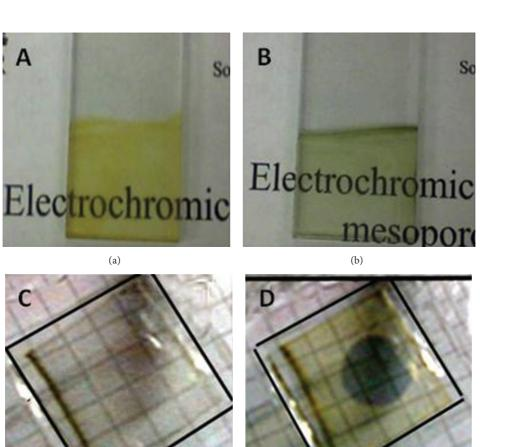
FIGURE 4: Electrodes appearance in electrochromic devices. (a) electrodeposited V2O5 on glass/ITO in the oxidized and (b) reduced form; (c) and (d) are respectively the bleached and coloured forms of the complete cell with sputtered WO<sub>3</sub> on ITO coated glass (cathode, working electrode) and V<sub>2</sub>O<sub>5</sub> on PET/ITO (anode, counter, and reference electrode).
