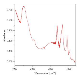
FIGURE 11: FTIR spectrum of V<sub>2</sub>O<sub>5</sub> film electrodeposited on ITO.
