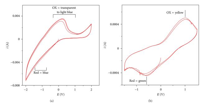
FIGURE 1: Typical CV of oxide films deposited on ITO prepared in this work. (a)  $WO_3/ITO$  cathode in LiNO<sub>3</sub> 0.1 M aqueous solution. (b)  $V_2O_5/ITO$  Anode in LiNO<sub>3</sub> 0.1 M ethanol solution. Electrodes configuration: ITO/Oxide film as working, Pt as counter, Sat. Ag/AgCl as reference. Scan rate 0.2 V/s. Color change is well visible by naked eye during scansion for both  $WO_3$  and  $V_2O_5$ . In the plots RED stands for reduced form and OX for oxidized form.
