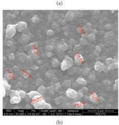
FIGURE 10: SEM pictures showing the high homogeneity and microporosity of  $V_2O_5$  film electrodeposited on ITO.
