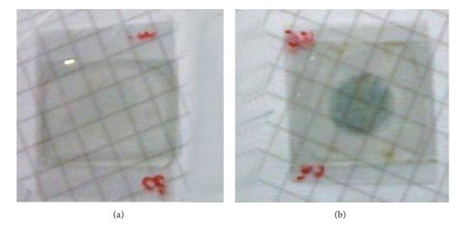
FIGURE 5: Single electrode EC device with BEMA/PEGMA electrolyte in bleached (a) and coloured state (b). Electrodes configuration: WO<sub>3</sub>/ITO/PET as cathode and ITO/PET as anode and reference electrode.
