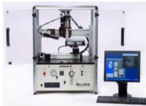
Figure 4.6 Ink Jet printer used for the experiments, with parameters fluid viscosity: 1-20 cP, drop volume: 10 pl 1 nl, nozzle diameter: 20-100 \mu\text{m} , drop velocity: 3 10 \text{ms}^{-1} .
