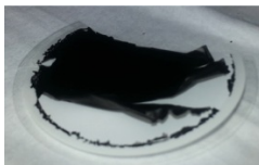
Figure 3.8 Picture of a freestanding rGO easily manageable flexible paper on an alumina filter for vacuum filtration.
