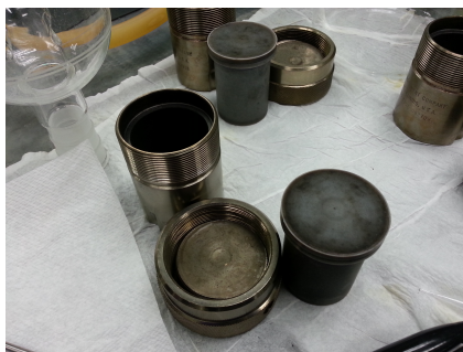
Figure 3.22 Picture of the Teflon-lined autoclave used for the hydrothermal synthesis.
