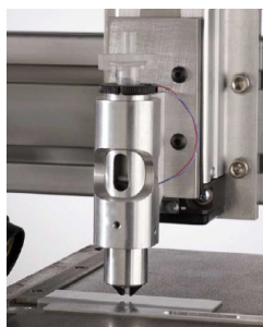
Figure 3.17 Image showing inkjet print head, printing on a glass slide.
