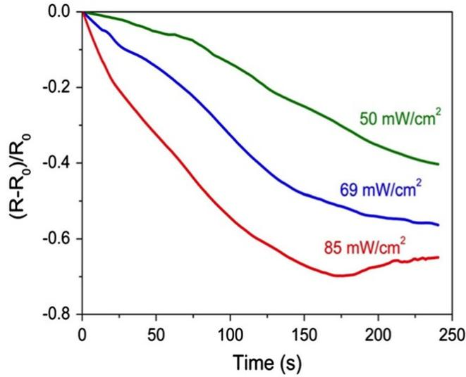
Figure 4.15 Real-time variation of PEGDA/GO resistance during UV irradiation, starting from as-printed non-polymerized material (time = 0), for three different UV light power densities
