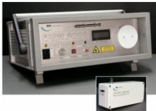
Figure 2.9. Main device and photodetector of the Fiber Optic Probe Hydrophone FOPH 2000
