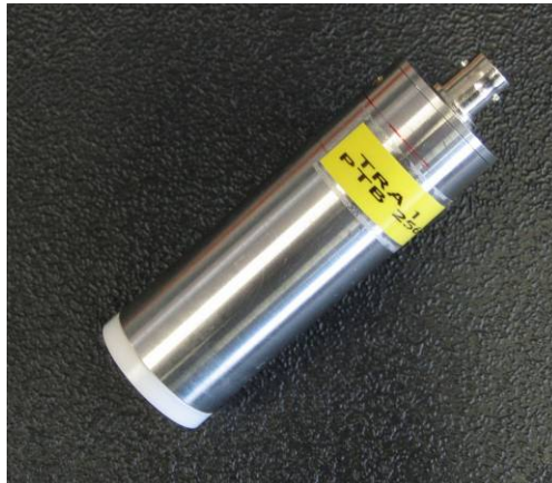
Figure 2.1. Transducer 1, PTB 256, piston-like
