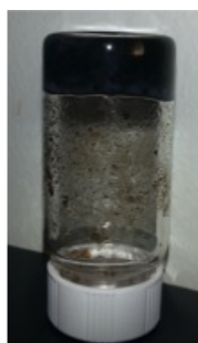
Figure 5.35 Sodium silicate gel with graphene oxide as a filler.
