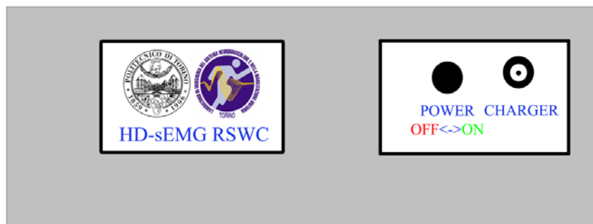
Figure3.8: Front panel (Panel A) of the HD-sEMG recording system with wireless communication (HD-sEMG RSWC) prototype. This panel includes the logo of HD-sEMG RSWC unit, power on/off switch and charger connector.
