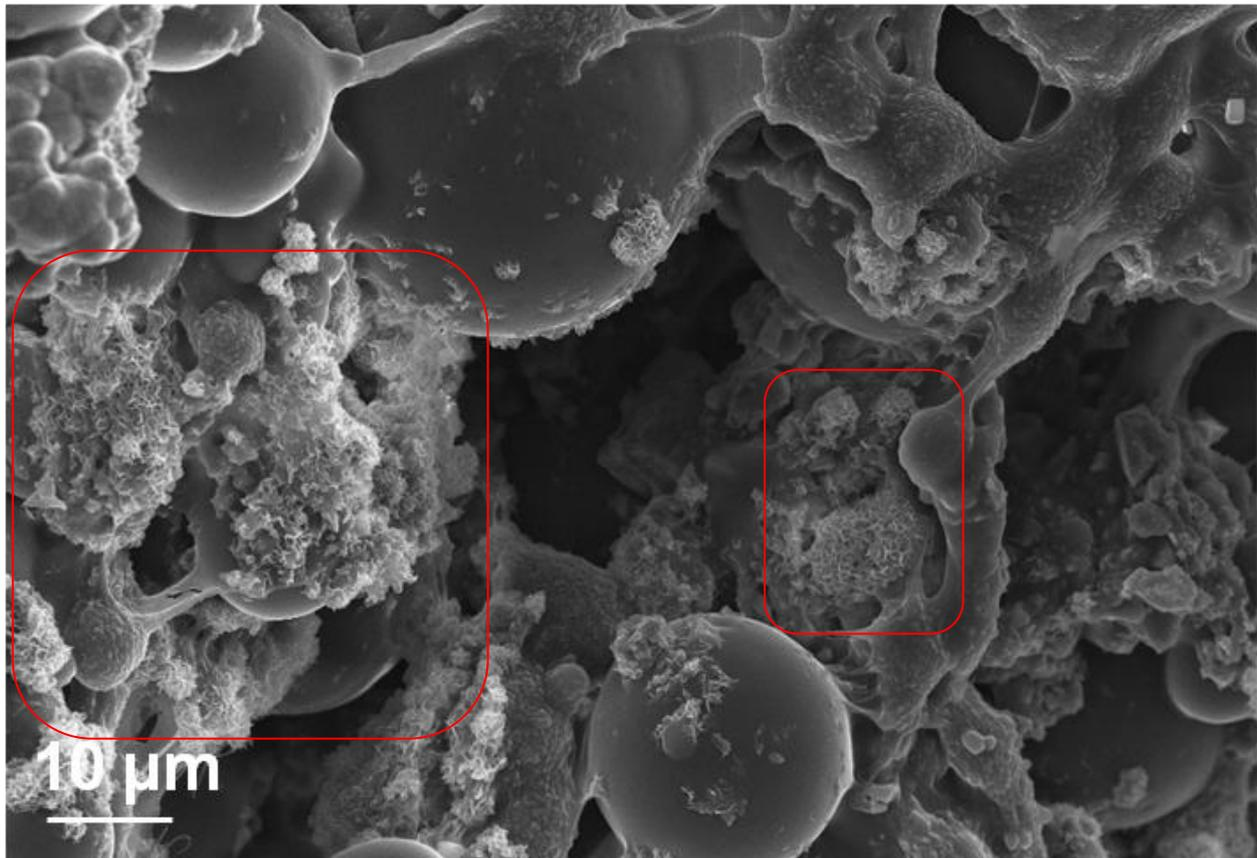
Figure 6.88: Morphology observations of precipitates on P15 cement after 72 hours of cultivation
