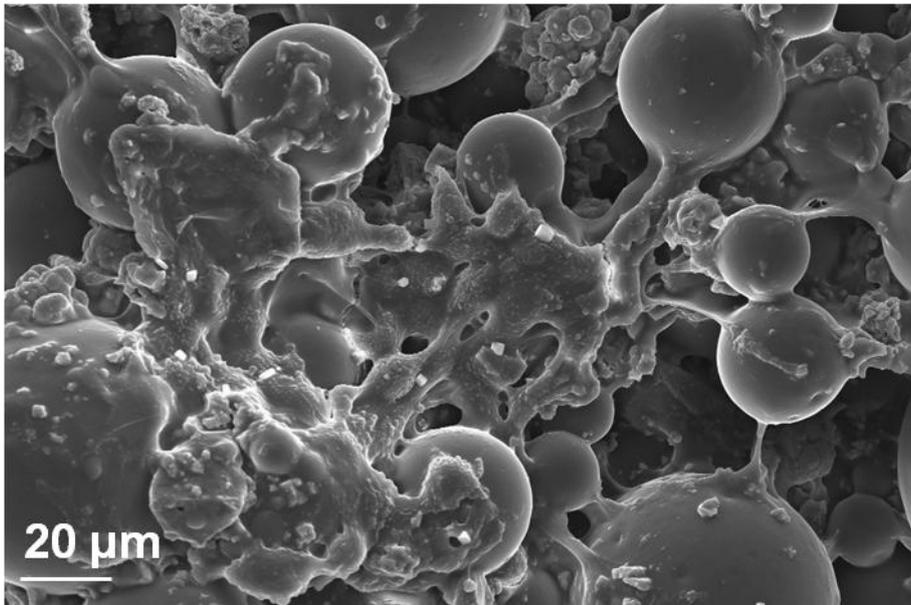
Figure 6. 78: Morphology observations of cells seeded on P15 cement after72 hours of cultivation
