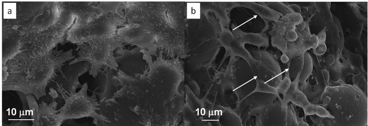
Figure 6. 67: Morphology observations of cells seeded on P10 cement after 72 hours of cultivation
