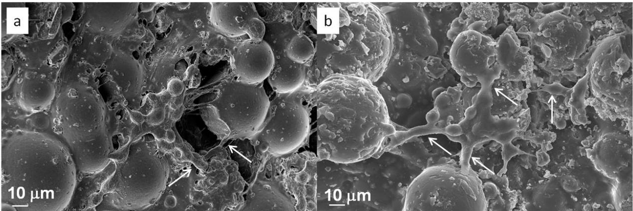
**Figure 6.55: FESEM morphology of cells seeded on P10 after 24 hours of culture**
