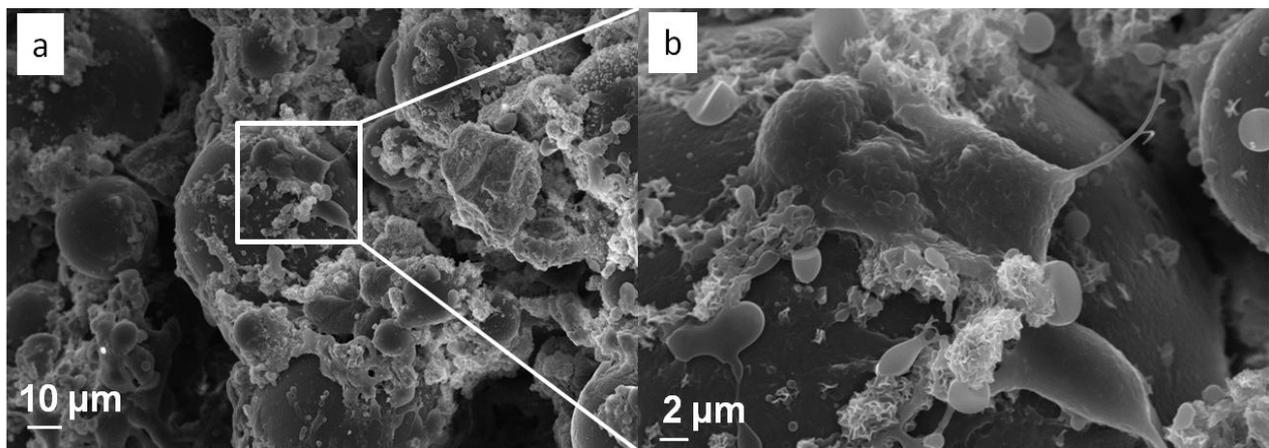
Figure 6.62: FESEM morphology of precipitates on P10 after 48 hours of cultivation
