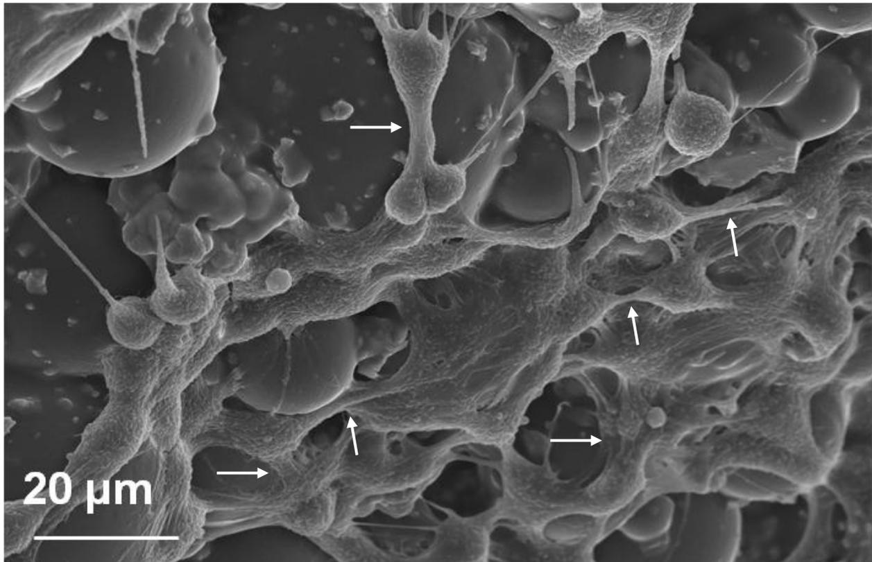
Figure 6.74: Morphology observation of cells seeded on P15 cement after 48 hours of cultivation
