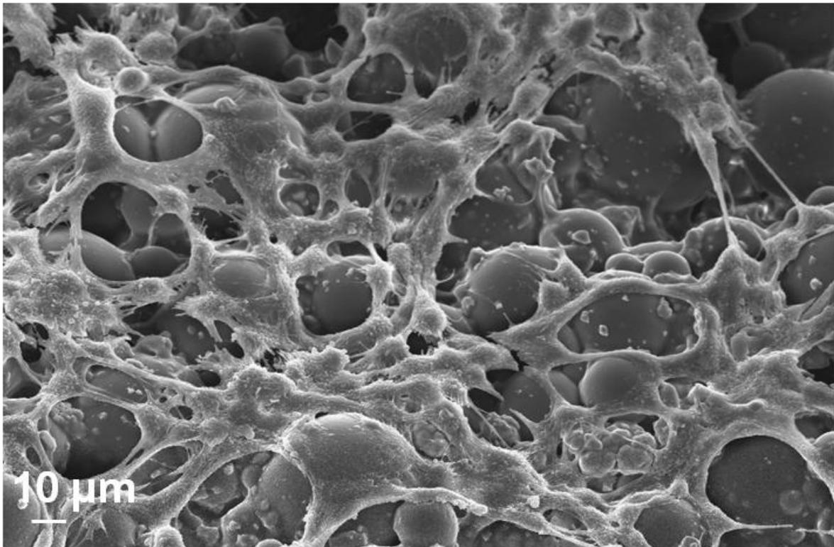
Figure 6. 76: Morphology observations of cells seeded on P15 cement after 48 hours of cultivation
