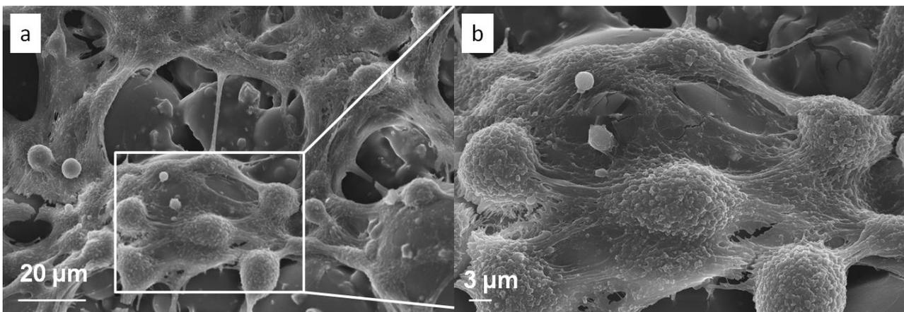
Figure 6.75: Morphology observations of cells seeded on P15 cement after 48 hours of cultivation
