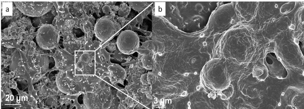
Figure 6.68: Morphology observations of cells seeded on P15 cement after 24 hours of cultivation
