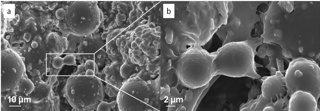
Figure 6. 90: Morphology observations of cells seeded on P20 cement after 24 hours of cultivation
