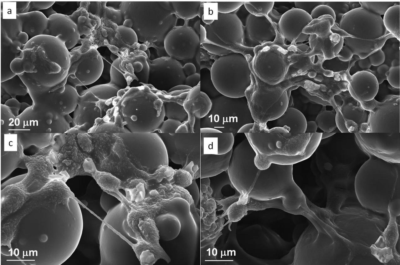
Figure 6.54: FESEM morphology of cells seeded on Palamed® after 72 hours of cultivation
