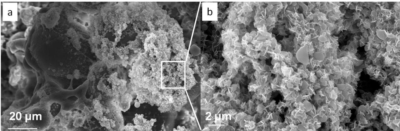
Figure 6.64: Morphology observations of cells seeded on P10 cement after 48 hours of cultivation.
