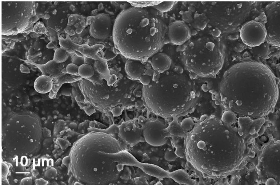
6. 91: Morphology observation of cells seeded on P20 cement after 24 hours of cultivation
