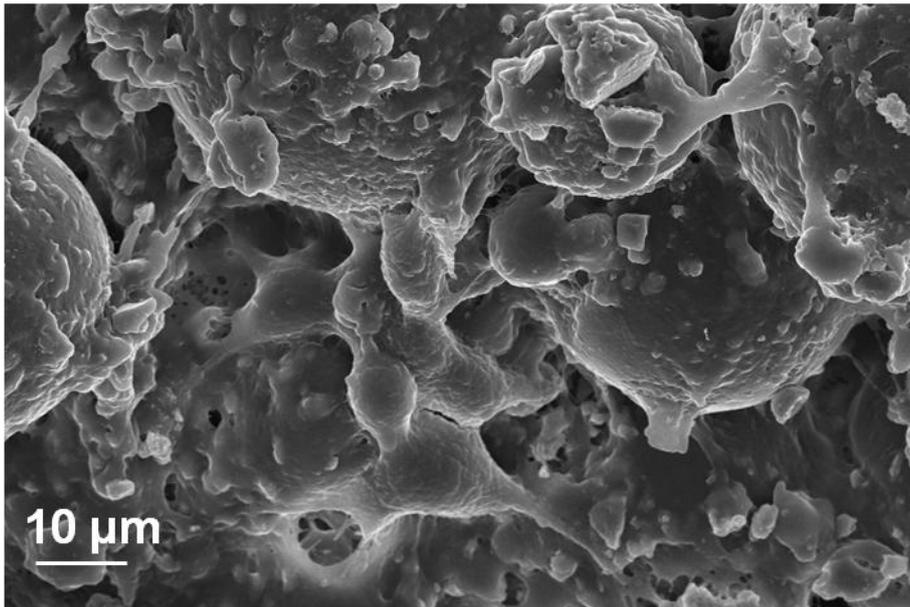
Figure 6. 97: Morphology observation of cells seeded on P20 cement after 24 hours of cultivation
