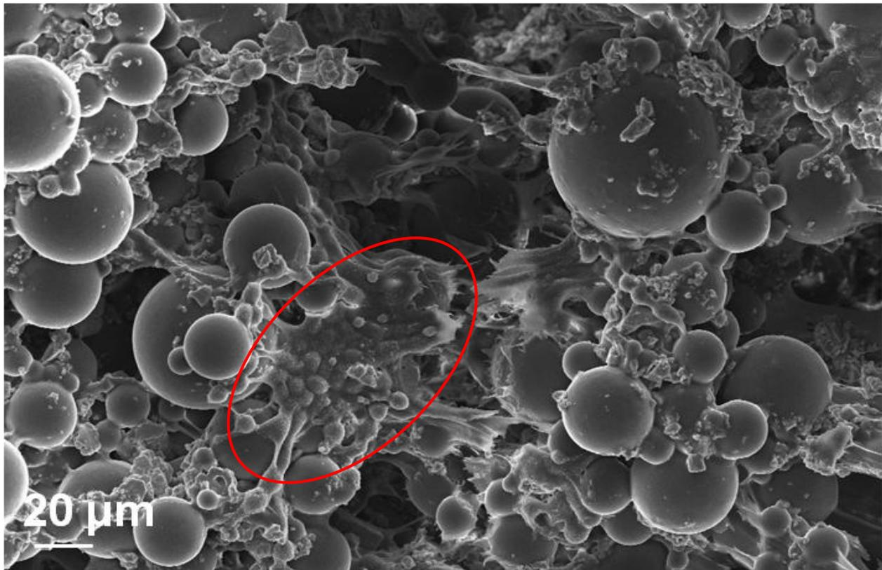
Figure 6. 79: Morphology observations of cells seeded on P15 cement after72 hours of cultivation
