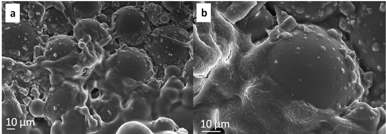
Figure 6. 101: Morphology observations of cells seeded on P20 cement after 48 hours of cultivation
