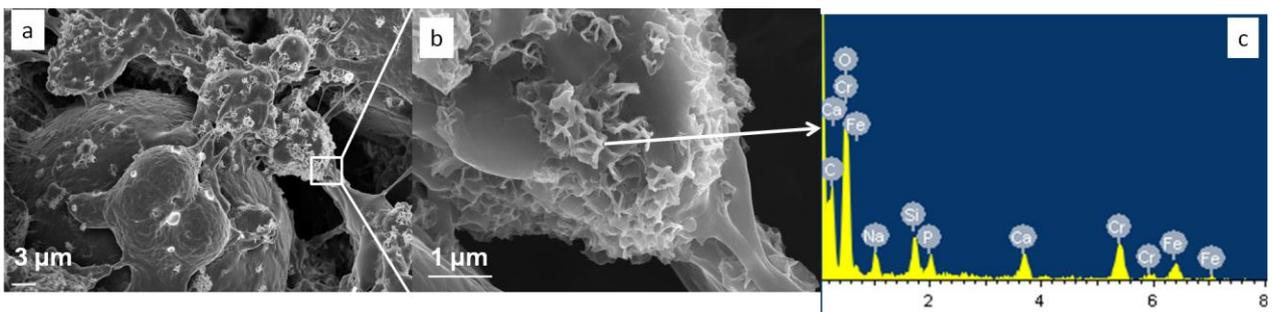
Figure 6. 81: Morphology observations of precipitates on P15 cement after 24 hours of cultivation
