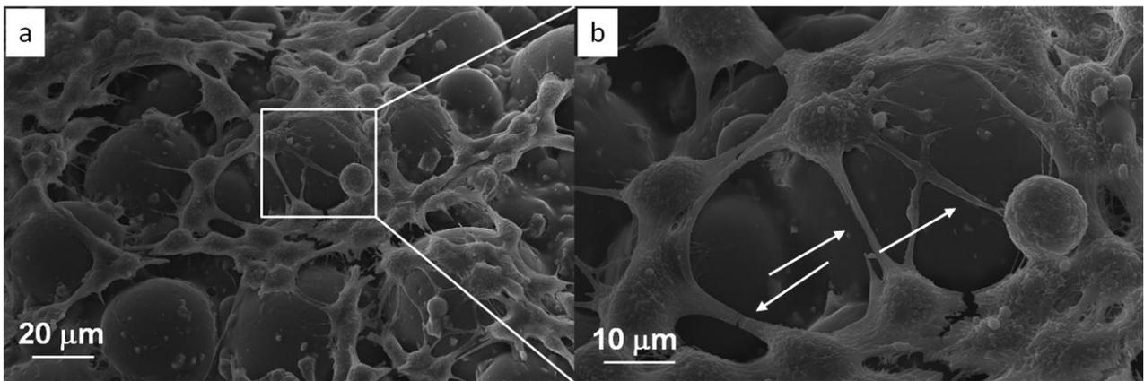
Figure 6. 66: Morphology observations of cells seeded on P10 cement after 72 hours of cultivation
