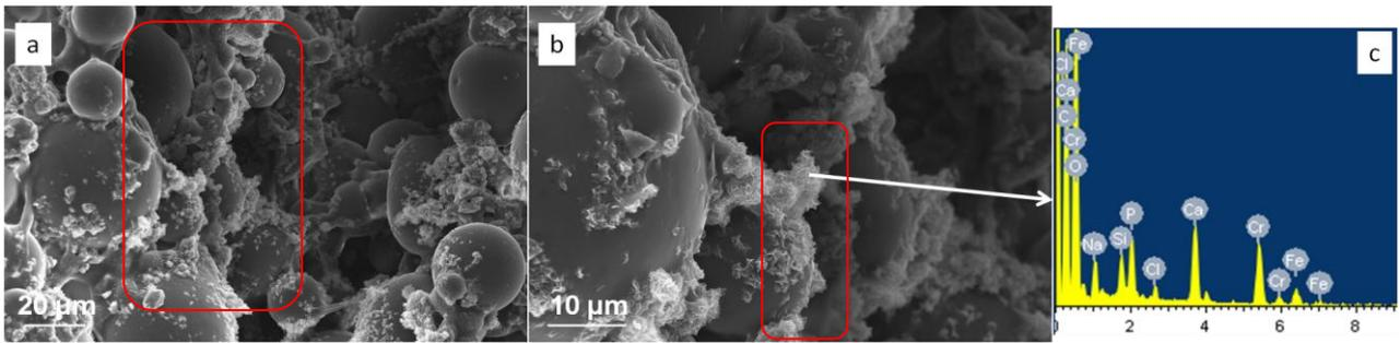
Figure 6.84: Morphology observations of precipitates on P15 cement after 72 hours of cultivation
