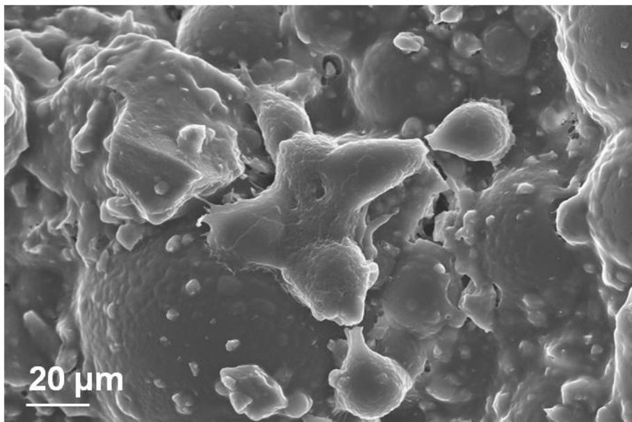
Figure 6. 103: Morphology observations of cells seeded on P20 cement after 48 hours of cultivation
