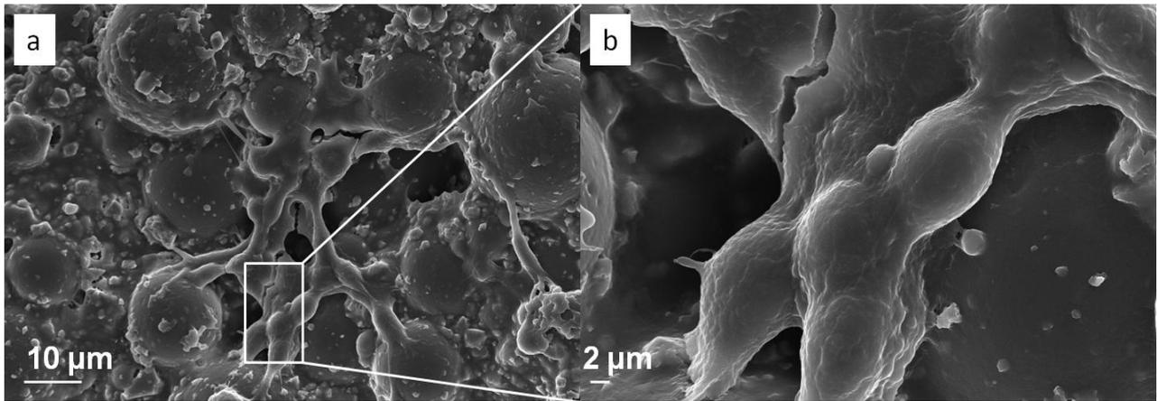
6. 92: Morphology observations of cells seeded on P20 cement after 24 hours of cultivation
