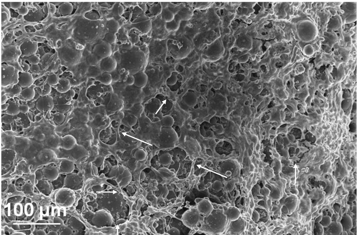
Figure 6.71: Morphology observation of cells seeded on P15 cement after 48 hours of cultivation
