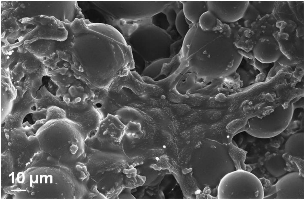
Figure 6. 80: Morphology observations of cells seeded on P15 cement after 72 hours of cultivation
