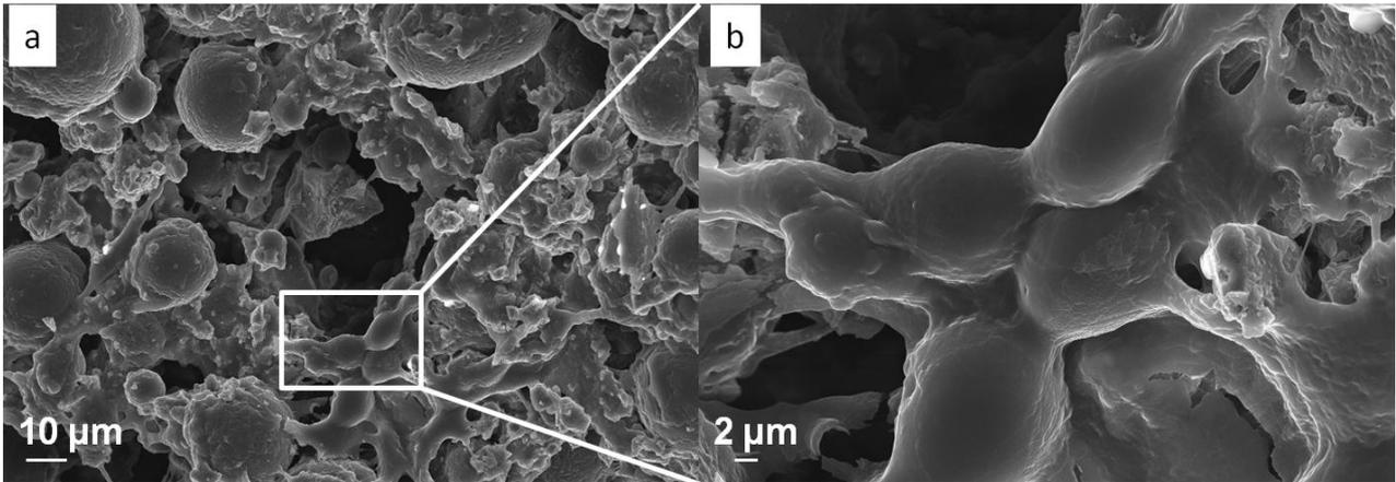
Figure 6.70: Morphology observations of cells seeded on P15 cement after 24 hours of cultivation
