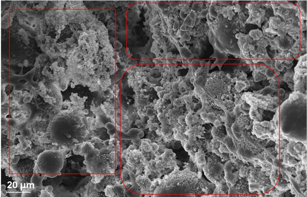
Figure 6.63: FESEM morphology of precipitates on P10 after 48 hours of cultivation
