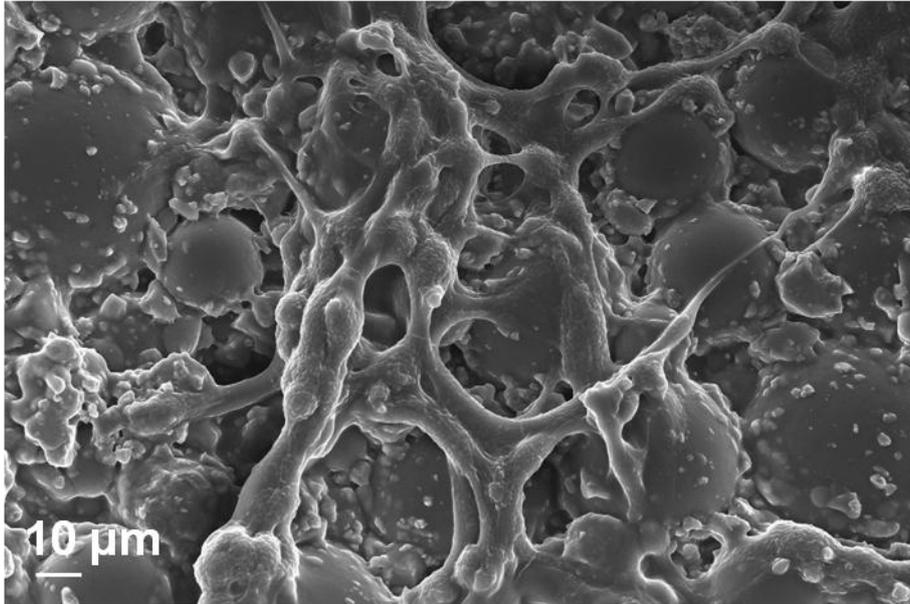
Figure 6.100: Morphology observation of cells seeded on P20 cement after 48 hours of cultivation
