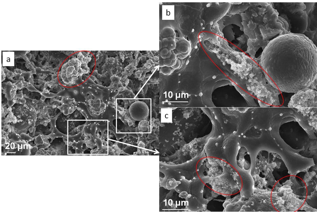
Figure 6.83: Morphology observations of precipitates on P15 cement after 24 hours of cultivation
