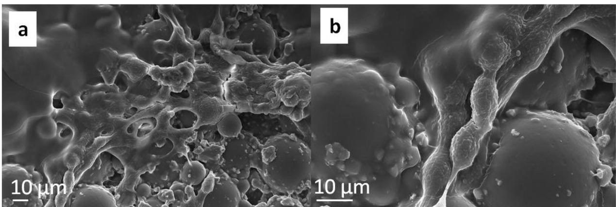
Figure 6. 99: Morphology observations of cells seeded on P20 cement after 48 hours of cultivation
