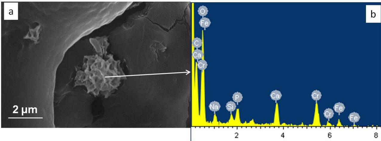
Figure 6.82: Morphology observations of precipitates on P15 cement after 24 hours of cultivation
