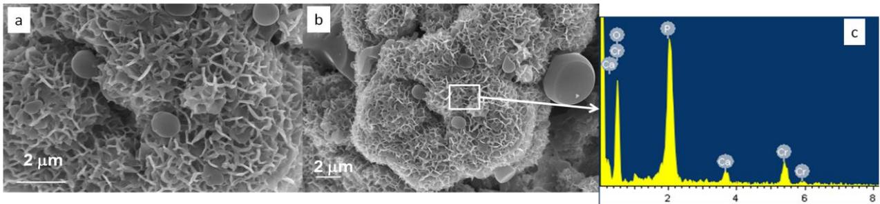
Figure 6.60: FESEM morphology of precipitates on P10 after 48 hours of cultivation
