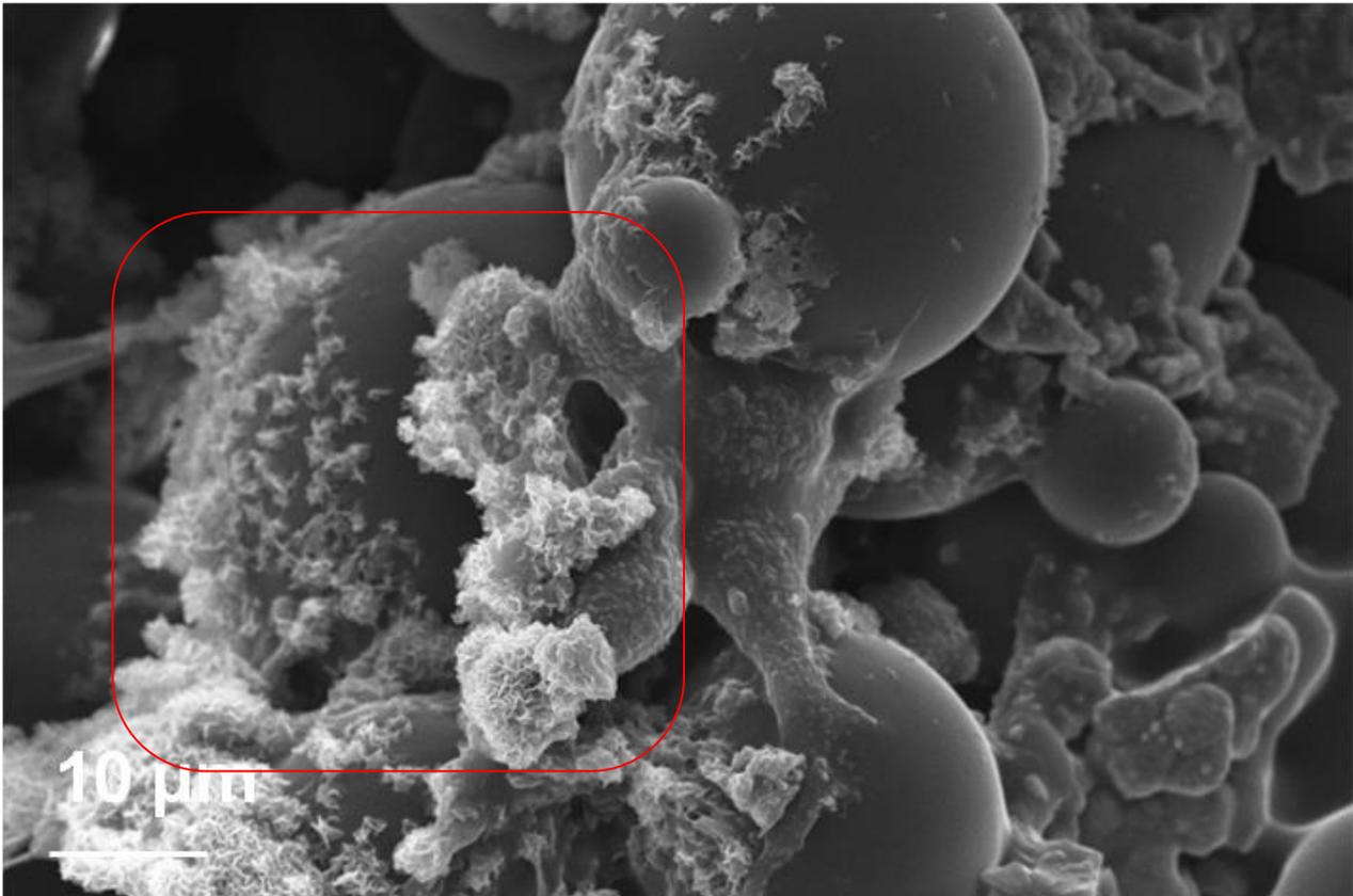
Figure 6. 87: Morphology observations of precipitates on P15 cement after 72 hours of cultivation
