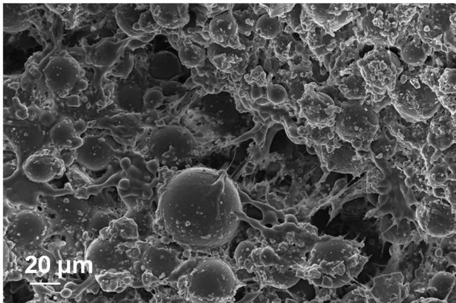
Figure 6.95: Morphology observations of cells seeded on P20 cement after 24 hours of cultivation
