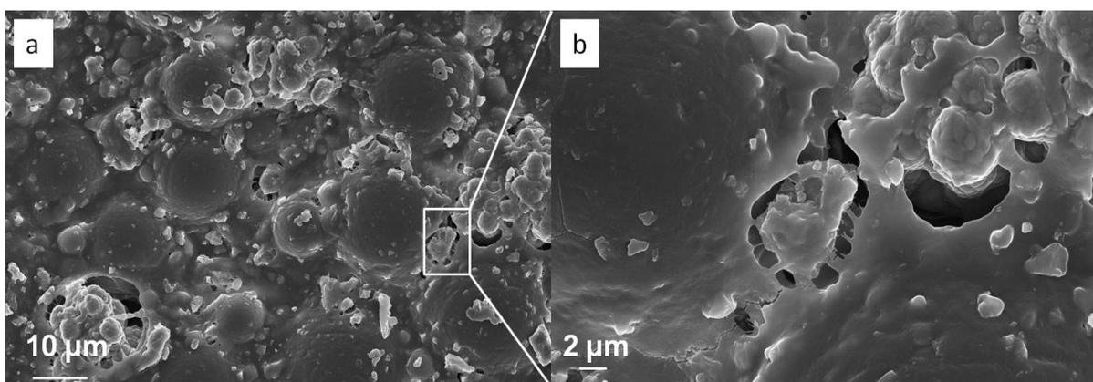
Figure 6. 96: Morphology observations of cells seeded on P20 cement after 24 hours of cultivation
