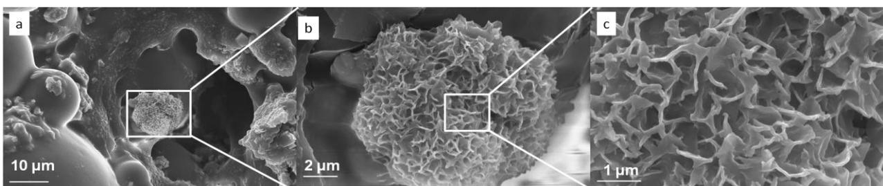
Figure 6.86: Morphology observations of precipitates on P15 cement after 72 hours of cultivation
