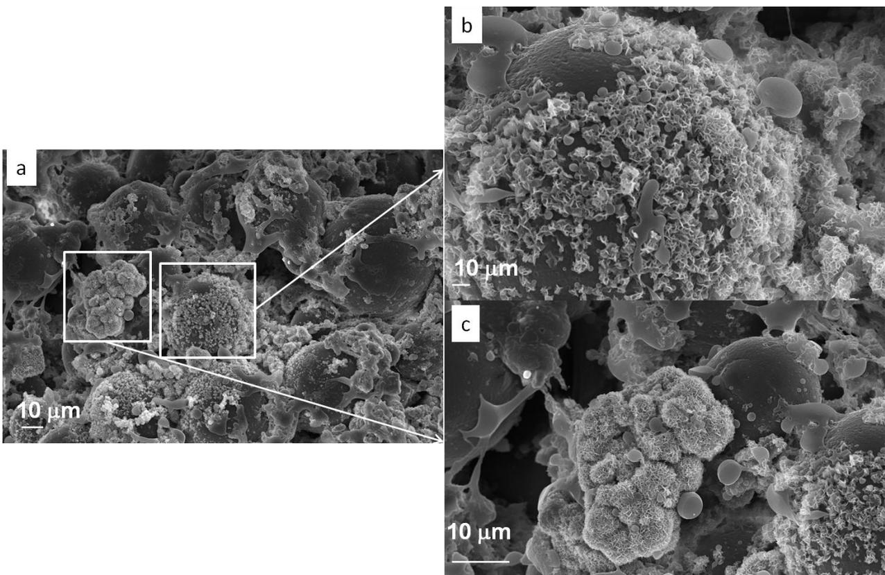
Figure 6.59: FESEM morphology of precipitates on P10 after 48 hours of cells cultivation
