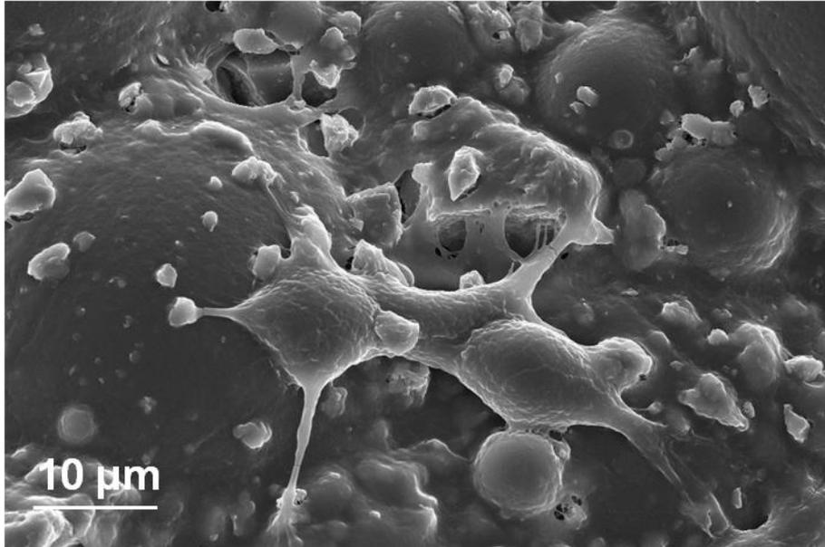
6. 90: Morphology observations of cells seeded on P20 cement after 24 hours of cultivation
