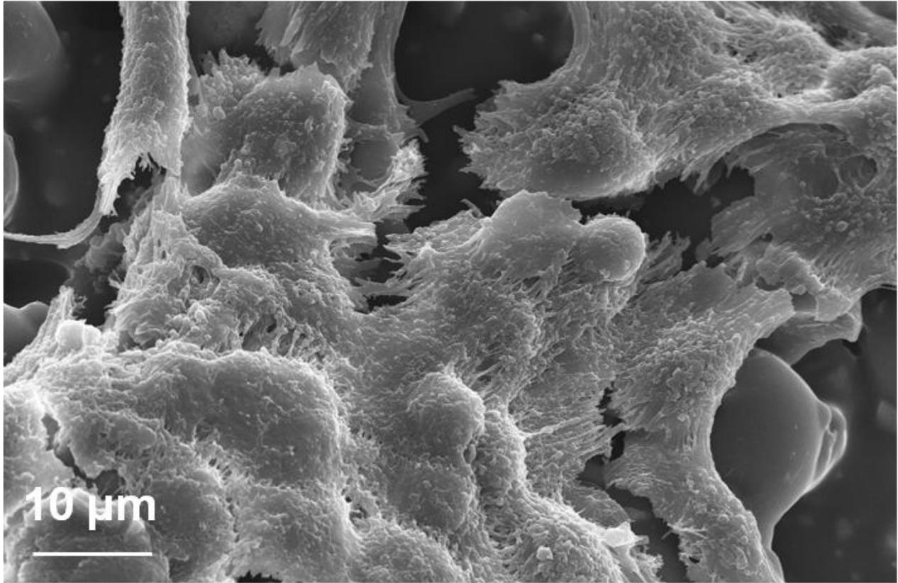
Figure 6. 72: Morphology observations of cells seeded on P15 cement after 48 hours of cultivation
