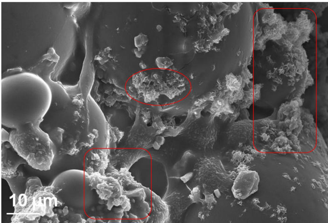
Figure 6.85: Morphology observations of precipitates on P15 cement after 72 hours of cultivation
