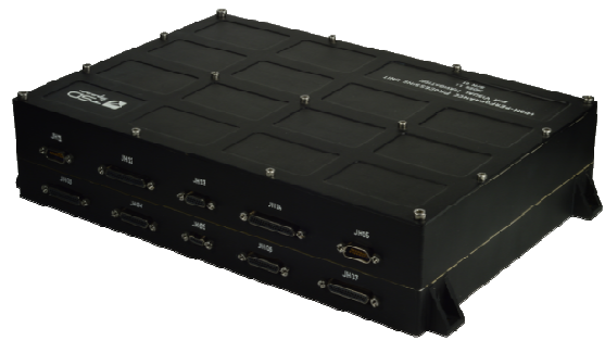
Figure 7: HPHC engineering model assembled in its cabinet
