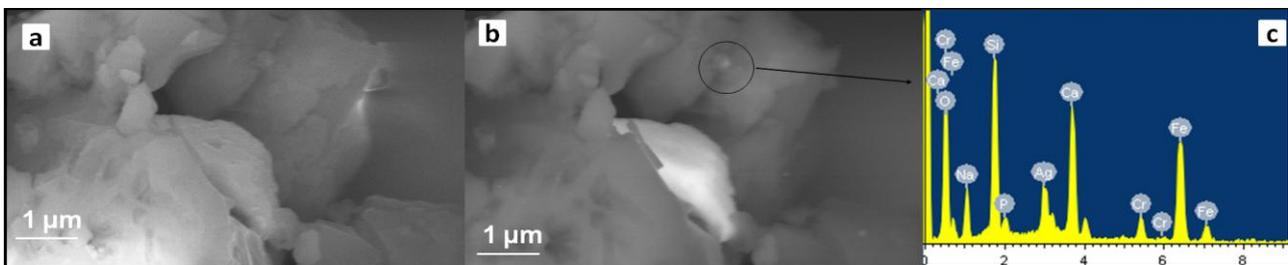
Figure 7.44: Morphology and compositional analysis of SC45 Ag2000
