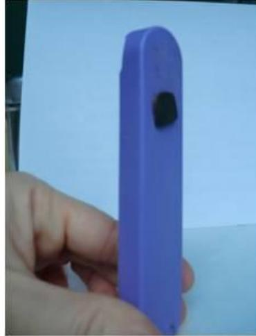
Figure 5.16: Magnetic interaction between a magnet and SC45-3Ag after annealing treatment
