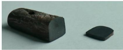
Figure 5.15: SC45-3Ag after annealing treatment at  $600^\circ\text{C}$  for 12 h
