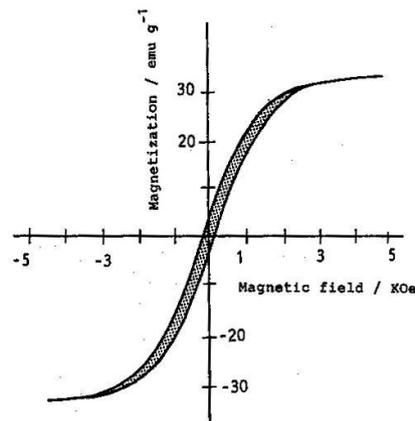
Figure 3.17: hysteresis loop of  $\text{CSFe}+\text{B}_2\text{O}_3+\text{P}_2\text{O}_5$  (CSFe+BP) glass heat treat at  $1050\text{ }^\circ\text{C}$  [13]
