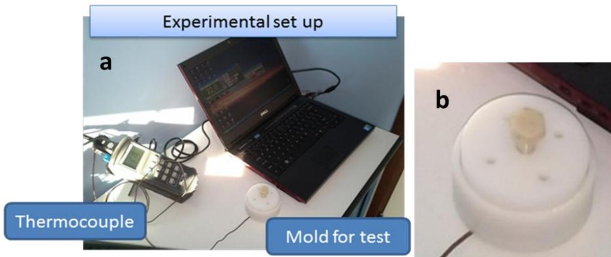
Figure 5.11: Experimental set up for setting time test in accordance with ISO 5822-2008.
