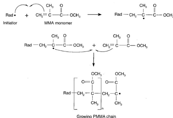
Figure 2.1: Polymerization of PMMA by an addition reaction. MMA monomer reacts with a radical to generate a second radical that can attack the double bond of another MMA monomer. [2]
