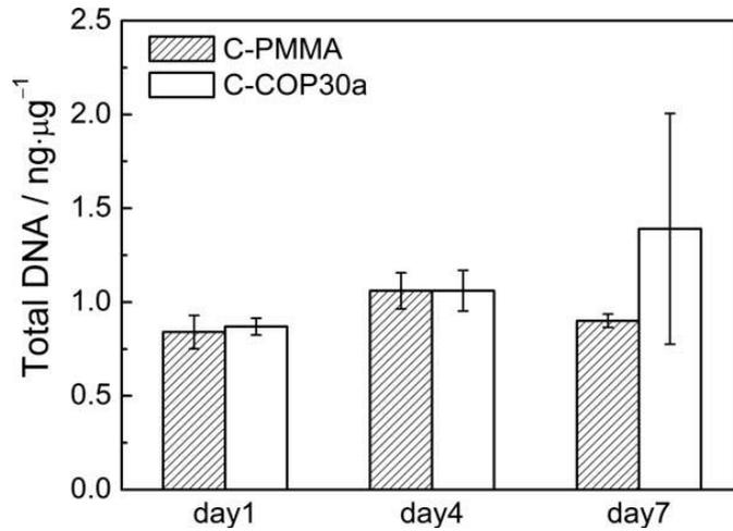
Figure4.6: The total DNA concentration of Rat-1 fibroblast cells adhered on cement discs. Data are shown as the mean  $\pm$  6 SD (n = 5).  $p > 0.05$  indicates no significant increases in the DNA concentration measured until day 7 of the culture for both types of cement discs.[2]
