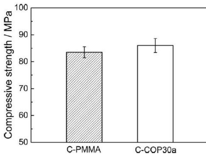
Figure 4.5: Compression strength without and with magnetite nanoparticles.[2]
