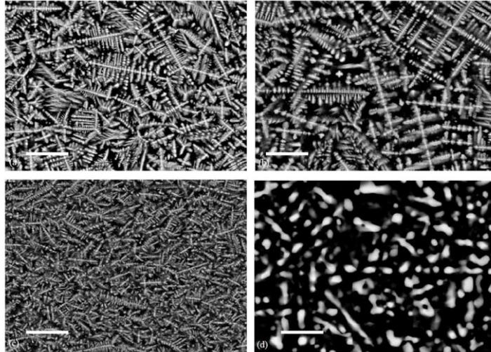
Figure 3.24: SEM images from samples of the series 20G presenting the effect of heat-treatment temperature on the microstructure of FBC: (a) as prepared, (b) heat-treated at 600 °C, (c) at 800 °C and (d) at 1100 °C. Bar is 2 mm.[18]
