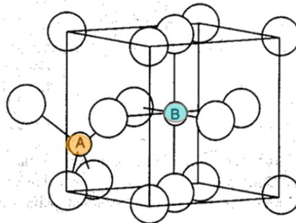
Figure 3.27: Tetrahedral and octahedral cation sites in the crystal structure of magnetite ( $\text{Fe}_3\text{O}_4$ ). In a tetrahedral site A the iron ion is surrounded by 4 atoms of oxygens while in octahedral site the iron ion is surrounded by six oxygen atoms. [10]
