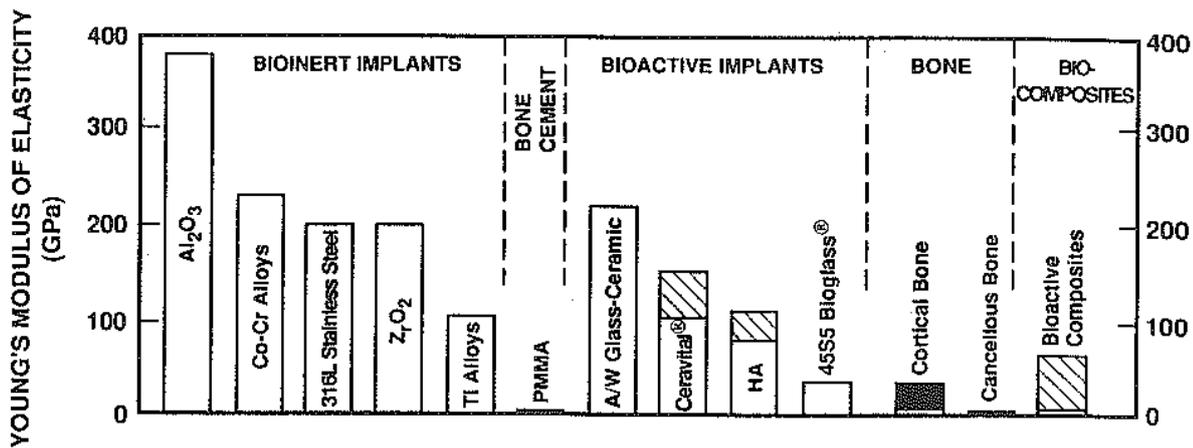
Figure 3.12: Modulus of elasticity (GPa) for prosthetic materials compared with bone[9]
