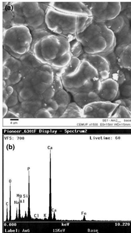
Figure 4.13: Ferrimagnetic cement immersed in normal SBF. A Precipitates covering the initial surface . b The precipitation of Ca and Mg phosphatate compound is detected. All the initial cement peaks of Si and Fe decreased and a high peak of P can be observed[7]
