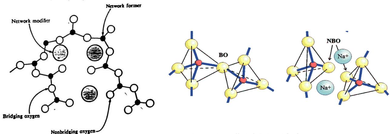
Figure 3.4: Glass structure: effect of alkali oxide[1,5]
