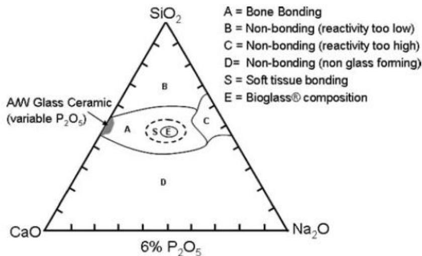
Figure 3.6: The graph shows compositional dependence (in weight percent, %wt) of the ternary compounds for the identification of the best bioglass formulation  $\text{P}_2\text{O}_5$  is constant at 6 %wt.[4]
