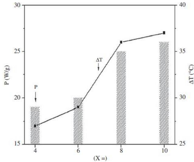
Figure3.21: variation of specific power loss and temperature as a function of iron oxide content.[17]
