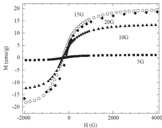
Figure 3.25: M–H plots of the samples with 5%, 10%, 15% and 20% molar fraction of Fe<sub>2</sub>O<sub>3</sub> in the reacting oxides. The response in applied magnetic field H up to 4 kG is shown.[18]
