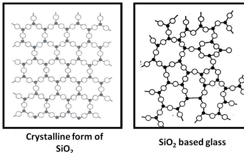
Figure 3.3: Difference between crystalline and amorphous SiO<sub>2</sub> [1]
