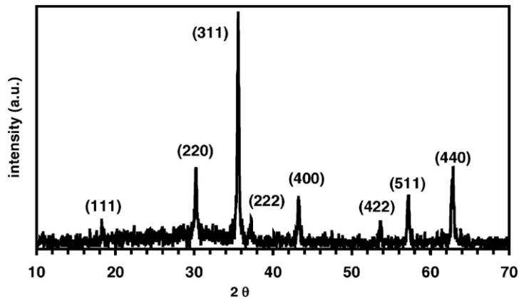
Figure 3.13: X-ray diffraction pattern (XRD) of glass ceramic[12]
