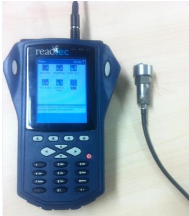
Figure 4.9- The data acquisition system and accelerometer used in the test rig.
