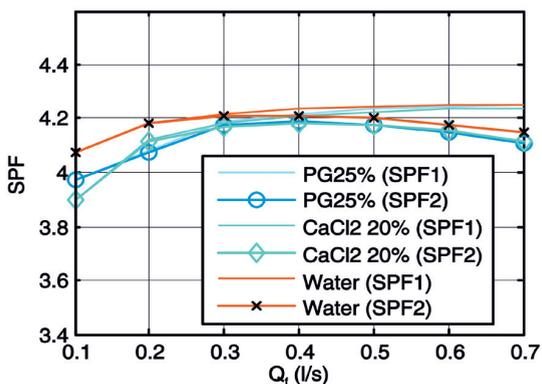
Fig. 3 – SPF<sub>1</sub> and SPF<sub>2</sub> for different heat carrier fluids and flow rates.
