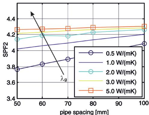
Fig. 2. GSHP Seasonal Performance Factor (SPF<sub>2</sub>) for different values of the pipe spacing and of the thermal conductivity of the grout (λ<sub>g</sub>).
