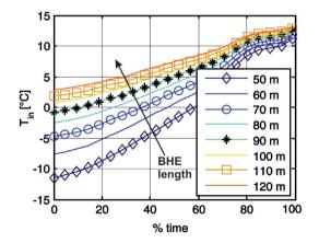
Fig. 1. Cumulate distributions of the inlet fluid temperature (T<sub>in</sub>) for different values of the BHE length.
