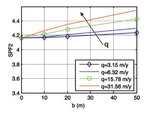
Fig. 5. SPF<sub>2</sub> for different values of the groundwater flow Darcy velocity (q) and of the aquifer saturated thickness (b).
