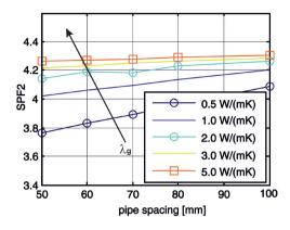
Fig. 2. GSHP Seasonal Performance Factor (SPF<sub>2</sub>) for different values of the pipe spacing and of the thermal conductivity of the grout  $(\lambda_g)$ .
