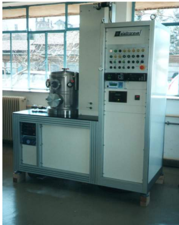
Figure 3.2. RF magnetron sputtering monotarget system.
