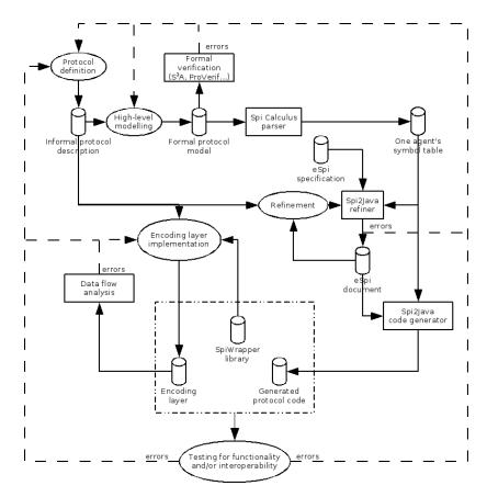
Figure 2.1: Spi2Java methodology workflow
