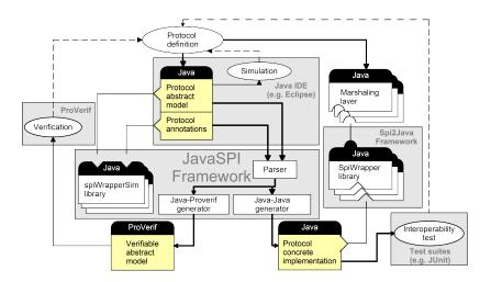
Figure 3.1: The complete workflow provided by JavaSPI
