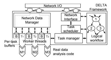
Figure 9.3: Architecture of the DELTA framework
