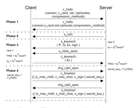
Figure 5.1: SSL message exchange in the selected scenario.
