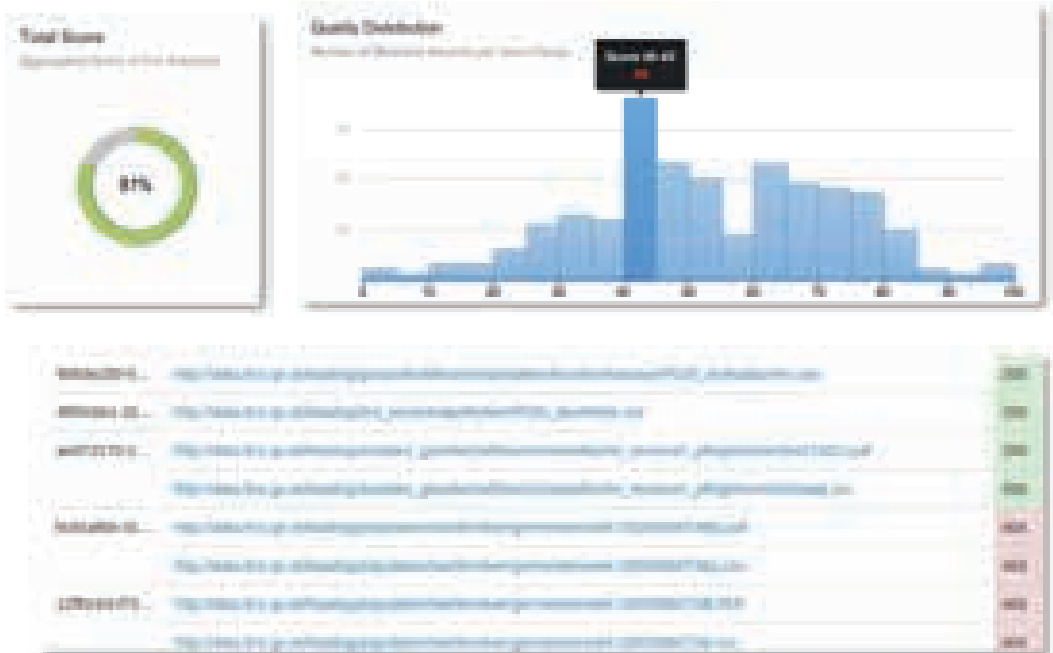
Figure 2: View components to communicate the results, e.g. metric score meter, quality score distribution (chart), link availability (table)
