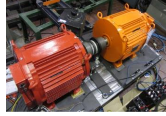
Fig. 14. Twin FASR prototypes, shaft connected on the test rig.
