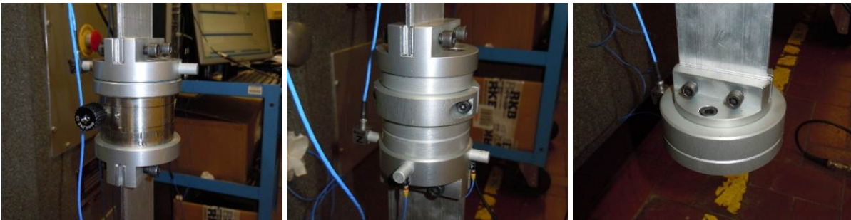
Figure 5.25 – Details of the test-rig: first added mass with rotating graduated device (left) second added mass with fixing device (middle) and third added mass (right).
