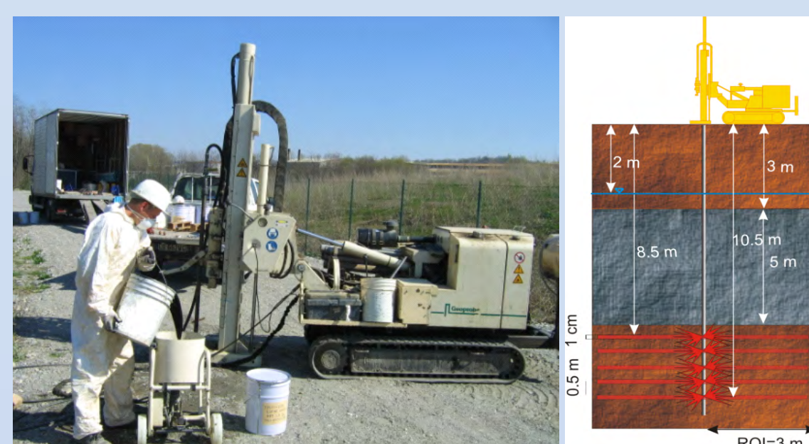
Field injection via direct push (cortesy of Carsico S.r.l., left) and scheme of stratigraphy and injection points (right)
