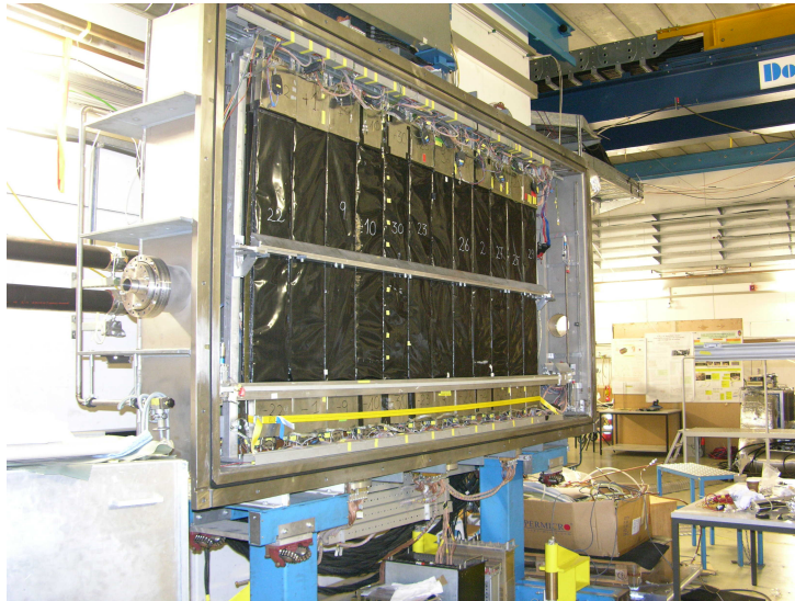
Figure 2.9: The ToF-Wall inside its slot.
