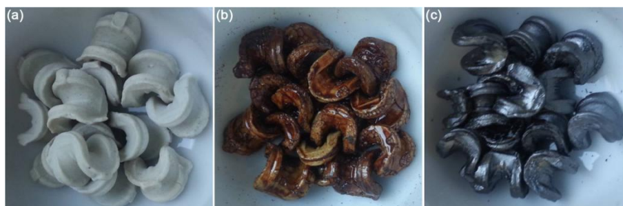
Figure 8.3. Image of the Berl saddles: (a) pristine (b) after caramelization (c) after pyrolysis of the glucose
