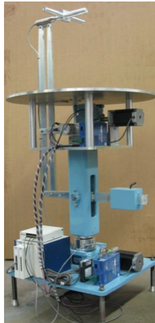
Figure 5.12: Clarkson University, Force/Moment Sting Balance and Model Positioning System
