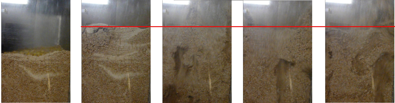
Figure 9.1: From left to right, first figure: initial condition potato-bran binary mixture, second figure: at minimum fluidization velocity, from third to fifth: fluidization at higher velocities (respectively, 2.2 u_{mfA} , 2.5 u_{mfA} , and 2.8 u_{mfA} approximately). Red line indicates the bed height at minimum fluidization velocity.
