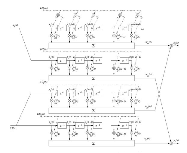
Fig. 4. Block diagram of the adaptive equalizer, including the updating rule: for example,  $h_{xx}^{(n+1)}(3) = h_{xx}^{(n)}(3) - \mu C_1 x_i^*(n-2)$ . The generation of coefficients  $C_1$  and  $C_2$  is shown in Fig. 5.
