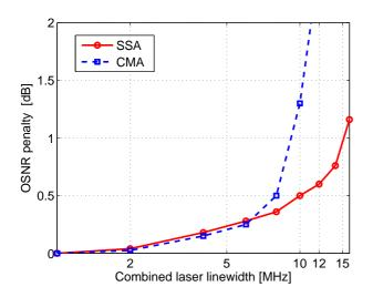
Fig. 8. OSNR penalty (at a reference BER equal to  $2 \cdot 10^{-2}$ ) vs. the combined laser linewidth.
