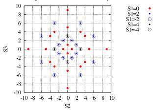
Fig. 3. Representation in the Stokes space of the ideal transmitted PM-16QAM constellation points for  $P_T = 5$ .
