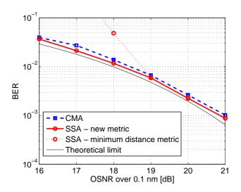
Fig. 6. BER vs. OSNR curve for buttery equalizer based on SSA and CMA update rules. The ideal theoretical curve is also shown as a reference.
