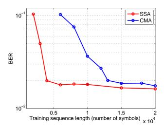
Fig. 7. BER vs. length of the training sequence (in number of symbols) for both SSA and CMA algorithm at OSNR=18 dB.
