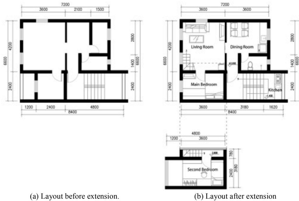
Fig. 26a, b: Area extension. The renovation was conceived to build an independent room for the son. As a result, the suite was finally changed to a duplex apartment. (Source: by author.)
