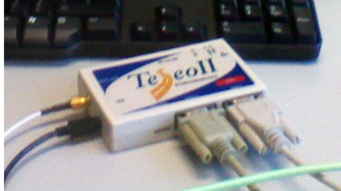
Figure A.5: The Teseo 2 evaluation board available at ESA ESTEC navigation lab.
