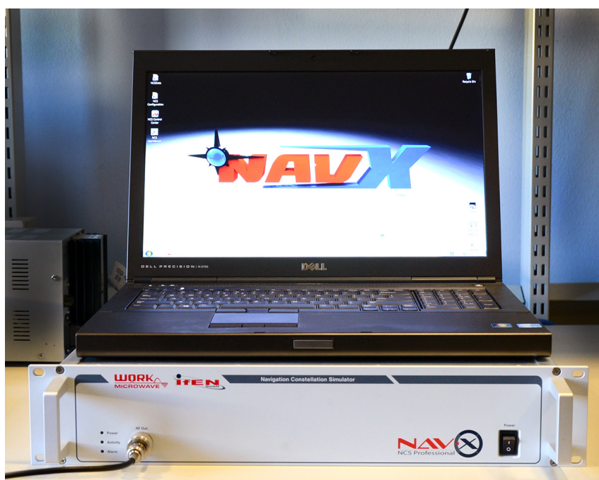
Figure A.4: The NavX NCS hardware signal generator available at ISMB navigation lab.
