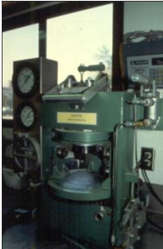
Figura 5.3.2.1: Il Texas gyratory shear test machine (1987)
