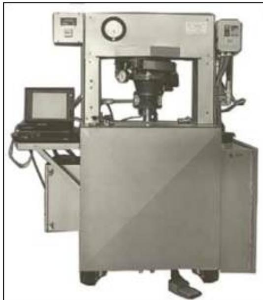
Figura 5.3.1.2: McRae e U.S. Army Corps of Engineers' Gyratory Kneading Compactor (anni '50)
