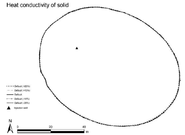
Fig. 13. Location of 16.0°C isotherms after 60 days of injecting warmer water for various values of solid thermal conductivity \lambda_s .
