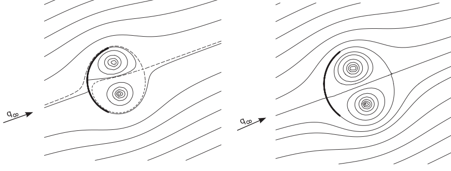
Figure 7. Circular arc at incidence ( \alpha = 20^\circ ). Left: \gamma_0 = 0 , \Delta\psi_{st} \neq 0 ; right: \gamma_0 = 0.18 , \Delta\psi_{st} = 0
