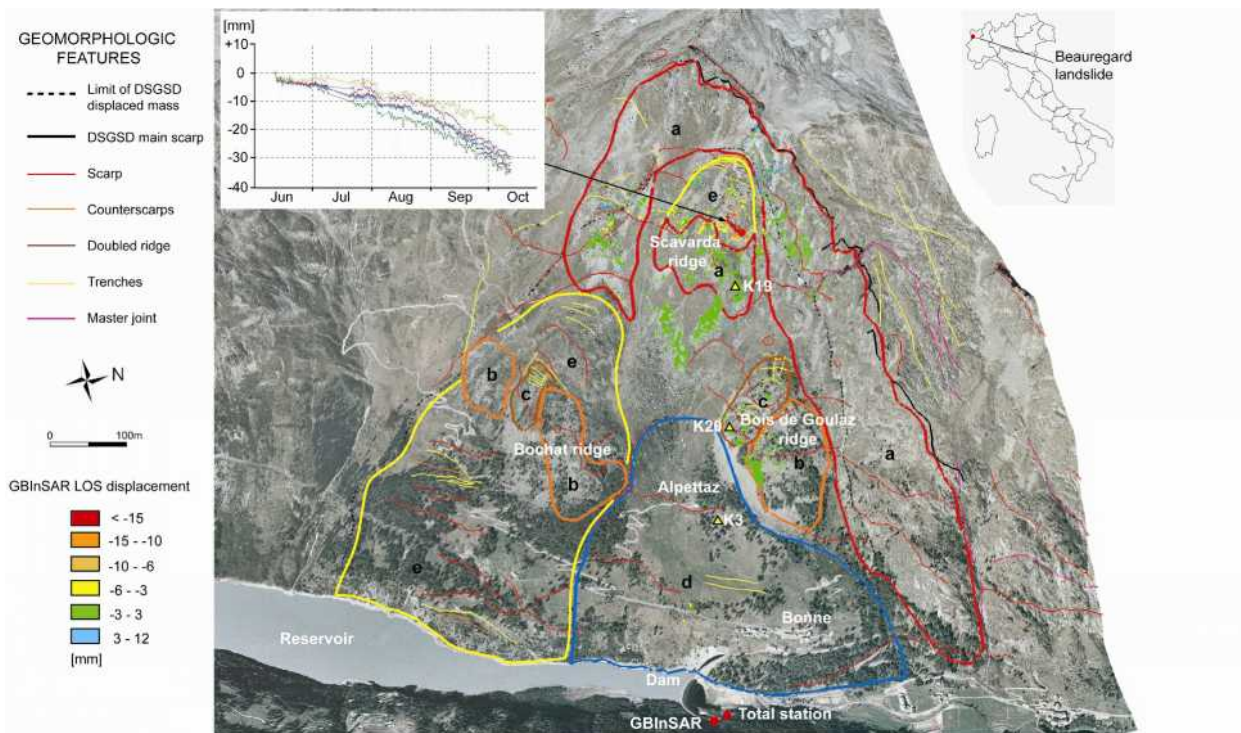
Figure 3. Beaugard landslide: results of the 2009 GBInSAR survey and geomorphologic features with indication of the main kinematic landslide elements : a) rock fall, b) block toppling, c) flexural toppling, d) slide on rotational surface, e) slide on compound surface.
