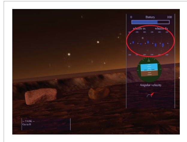
Figure 10. Highlighted Skid events indicator on left screen.
