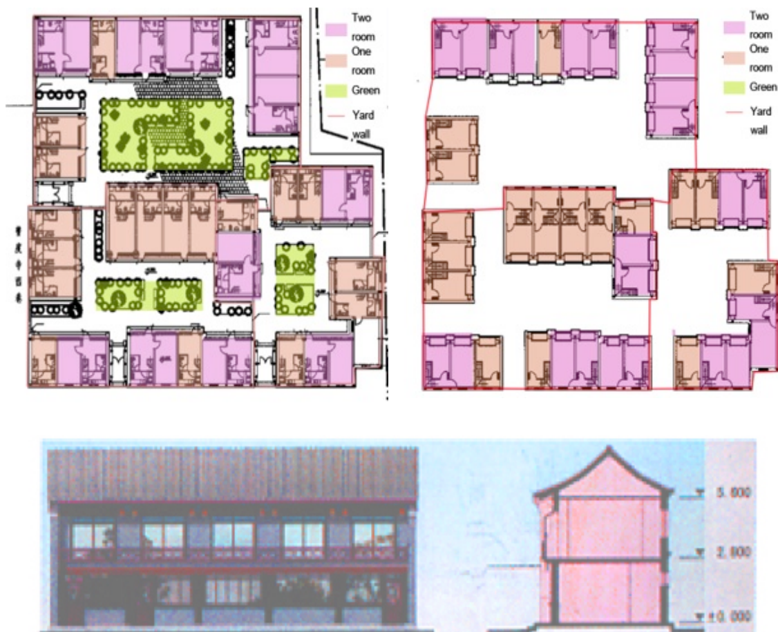
Figure 1-49: The storied-courtyard building plot, facades and sections
