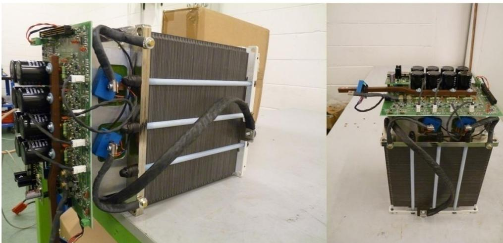
**Figure 4.4.** Picture of the first prototype implementing the DC-DC thermal and electrical integration with the stack.
