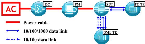
Fig. 1. Experimental testbed for power measurements, inclusive of AC power supply (AC), optional DC power supply (DC), power meter station (PM), system under test (SUT), PC traffic endpoints (PC TE), and Spirent SmartBit SMB-200 traffic endpoints (SMB TE).
