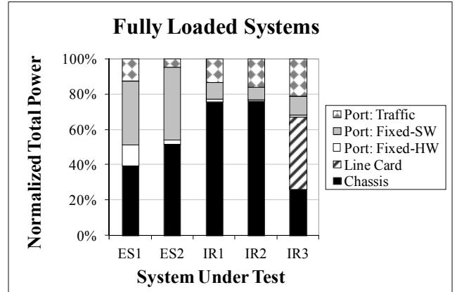
Fig. 2. Estimated breakdown of system power when all ports in the system are fully loaded. The port-traffic quota alone defines the current PTRA margin for saving energy. The port traffic and fixed-software quotas define the DTRA margin.
