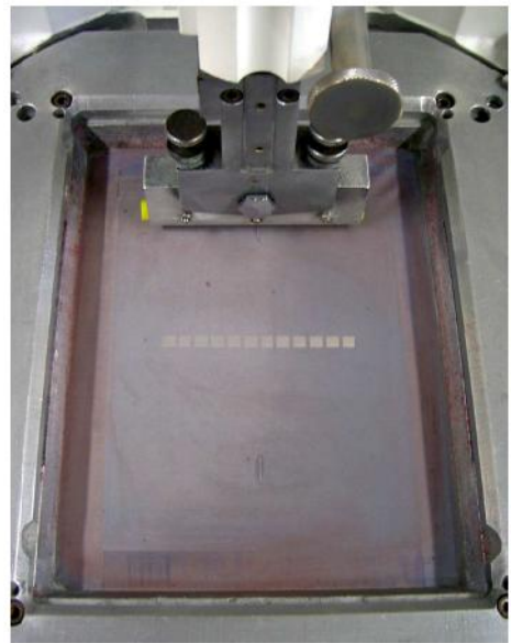
Figure 3.2.1.5. Patterns of the screens used to deposit a) the electrodes and b) the rectangular sensing films.
