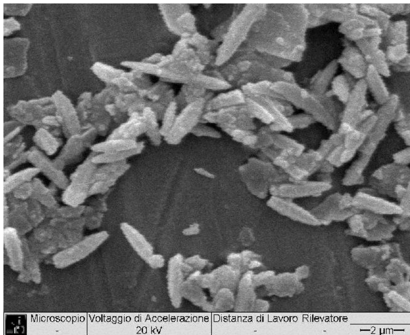
Figure 3.5.1.2. SEM analysis of ZnO nanopowder from hydrothermal synthesis in becker at 95°C for 90 minutes.
