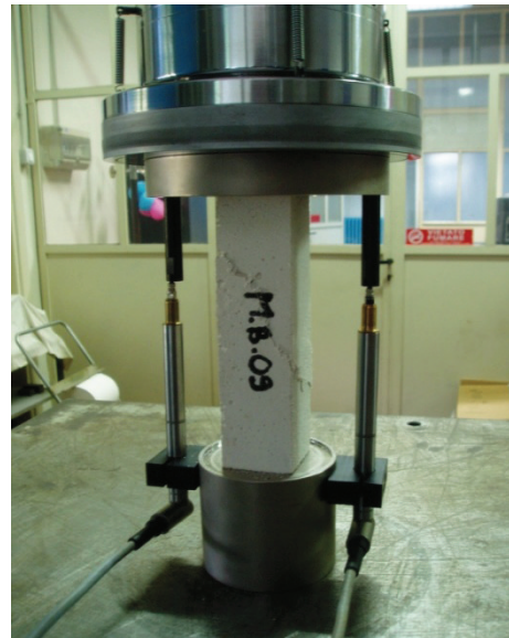
Fig. 5 Compression test on single mortar specimen.
