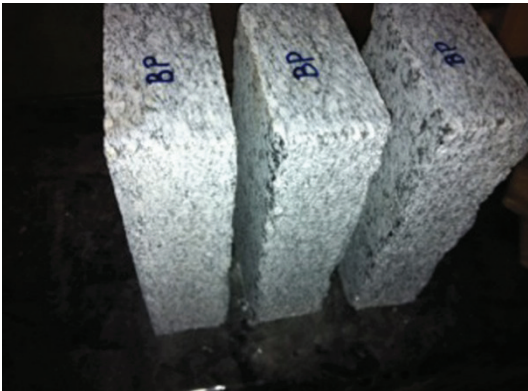
Fig. 8 Adherence surface of stone treated by pneumatic drill.
