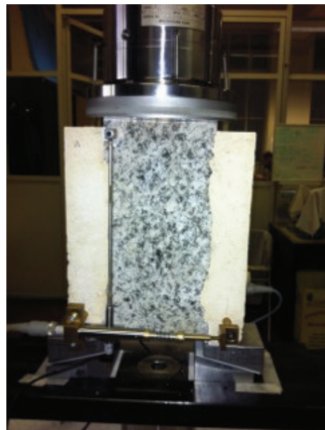
Fig. 10 Composite specimen stone-repair mortar.
