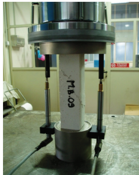
Fig. 5 Compression test on single mortar specimen.
