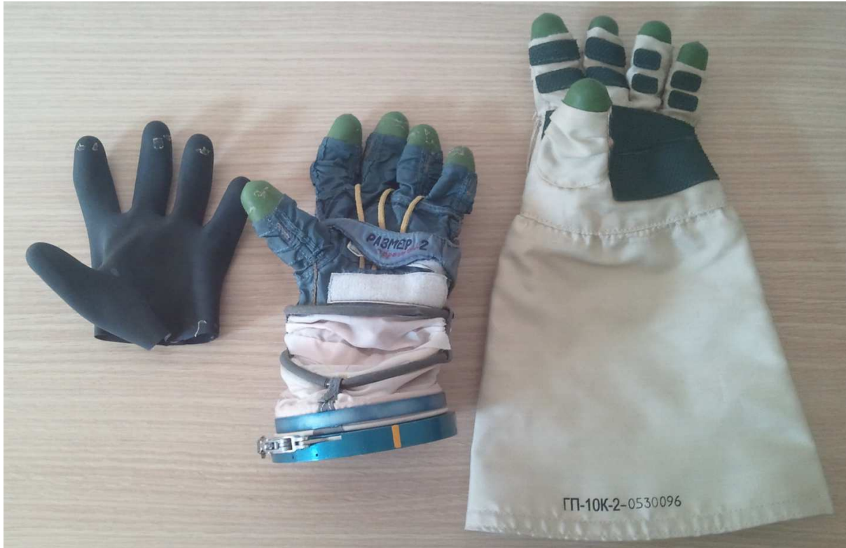
Figure 46: Three elements of Orlan-DM EVA glove; from left to right: bladder, restraint, ITMG
