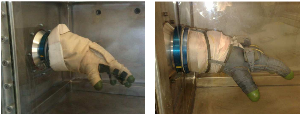
Figure 50: The Orlan-DM EVA glove inside the custom-made glove box with ITMG (left) and without ITMG (right)
