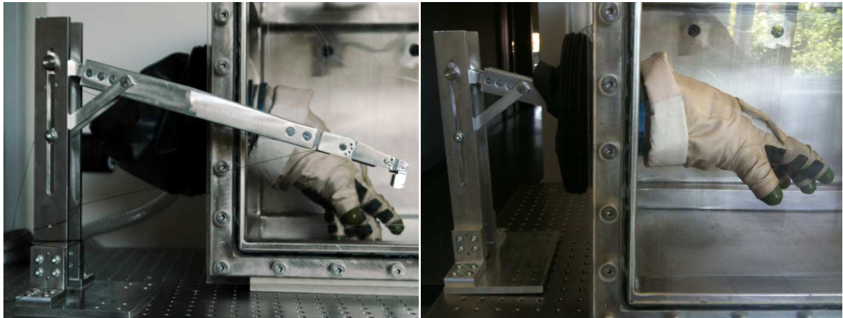
Figure 84: Finger probe in front and inside the glove box
