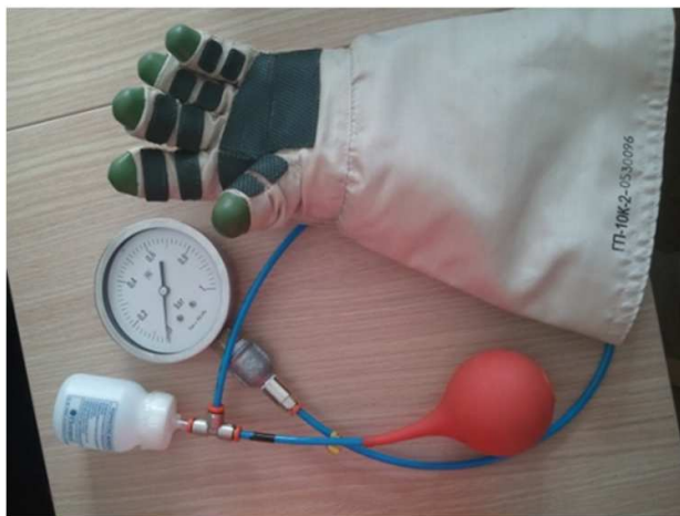
Figure 52: Home Made Measurement Setup outside (Left) and inside (Right) the Glove Box
