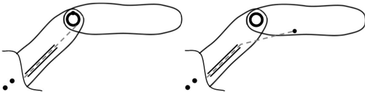
Figure 102: Wire actuation with (left) and without (right) access to the joint
