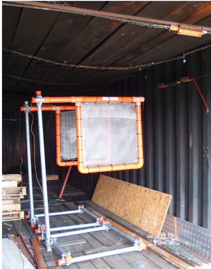
Figure 15. Targets used for wide fog measurements
