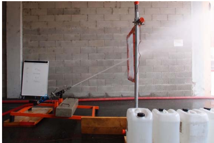
Figure 3. 'Branchpipe' experimental set-up
