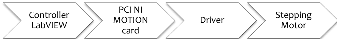
Figure II.7. Schematic diagram of the control subsystem components and their mutual connections.
